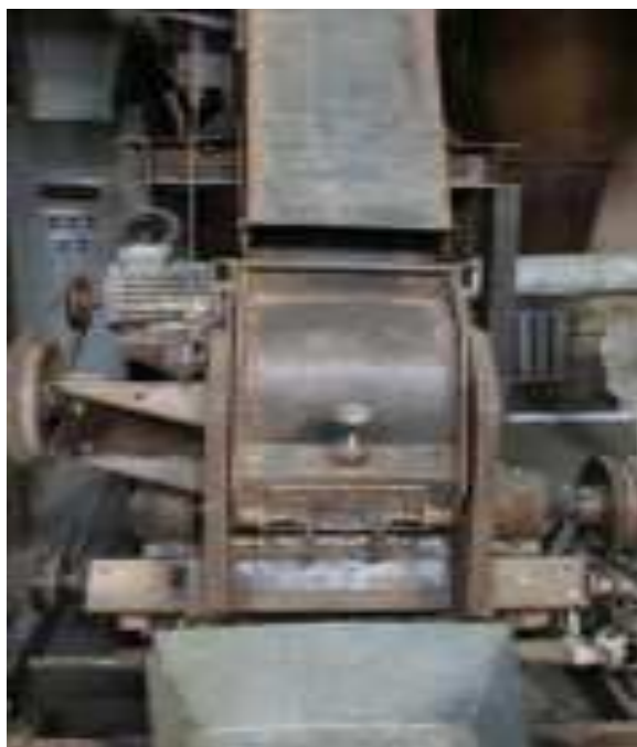
Figure 5. Working chamber 30 saw linter 5LP
