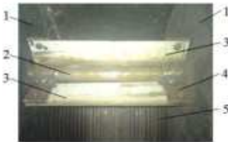
Figure 7. Working chamber 30 of the saw linter with a modernized agitator 1 - working chamber, 2 - blade, 3 - cross, 4 - shaft, 5 - sheet
