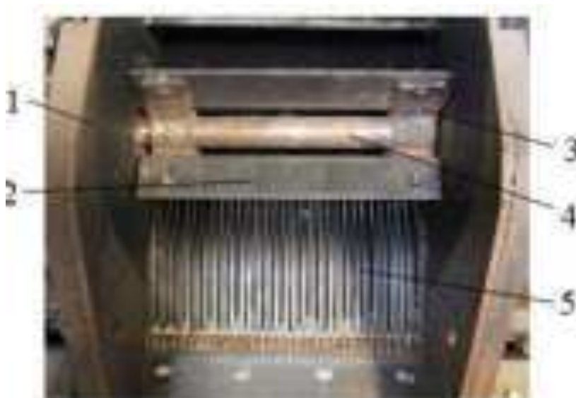
Figure 6. Working chamber 30 of the saw linter with a serial turner 1 - working chamber, 2 - blade, 3 - cross, 4 - shaft, 5 - saw cylinder.
