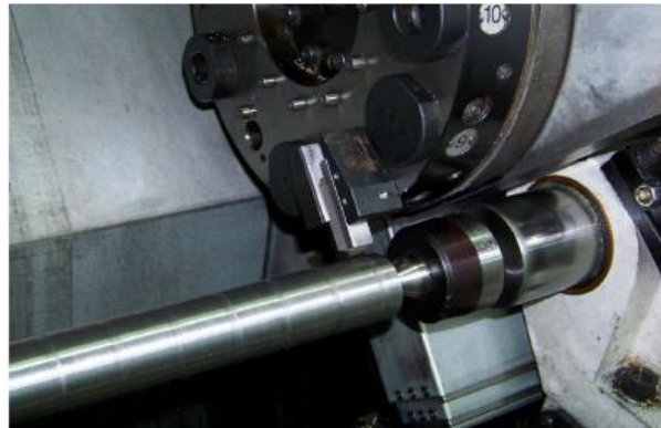
Figure 6. Photograph of the workpiece processing area on a V turn 20 CNC lathe.
