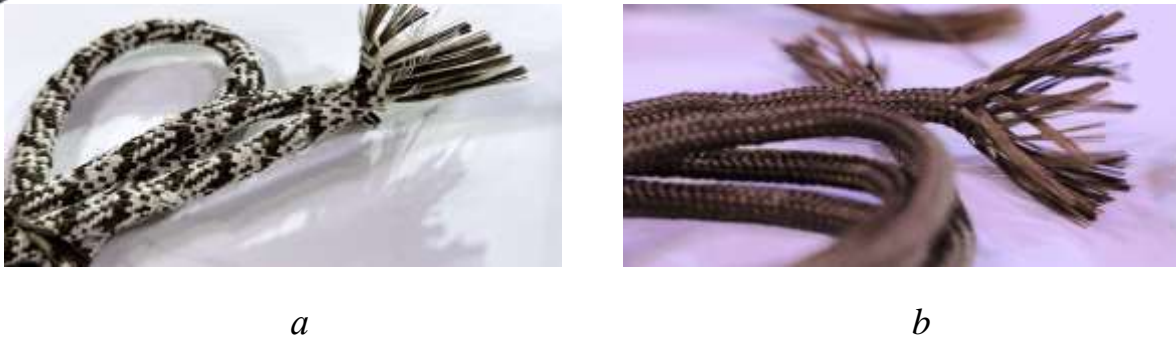
Figure 2. Cord view: a - cord from basalt and cotton thread; b – basalt cord
