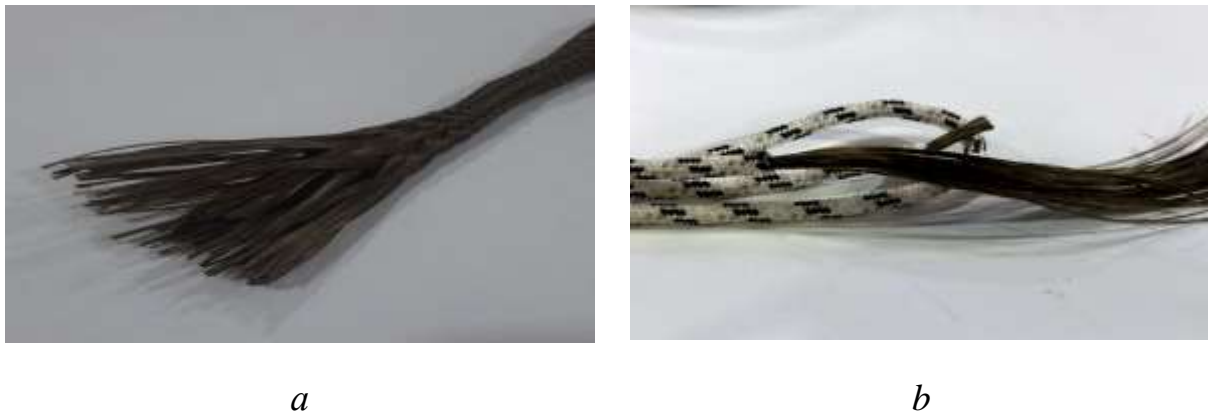
Figure 2. Cord view: a - cord from basalt and cotton thread; b – basalt cord
