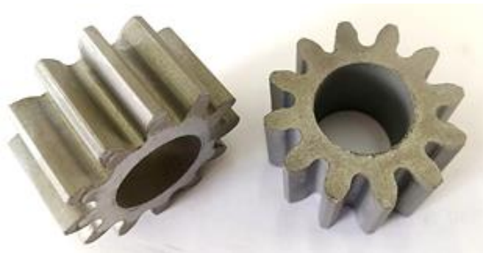
Figure 2. Gear wheel parts that have undergone the heating and baking process.
