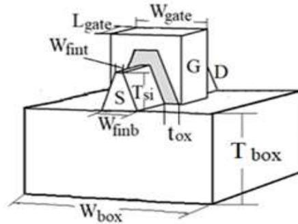
**Figure 1. The geometric structure of the modeled vertical field-effect transistor**
