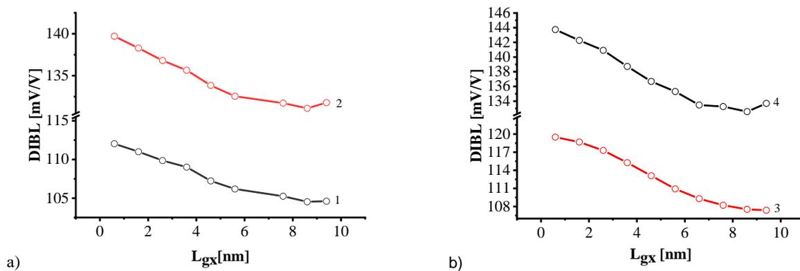
**Figure 2. For the two cross-sectional forms of the DIBL effect, the position of the single charge channel covered at the oxide-semiconductor boundary between the roof and the side surface along the channel is related to  $L_{gx}$  a) between the roof surface of the covered single charge channel, 1- trapezoidal 2-rectangular cross-sectional transistors b) 3-trapezoidal 4-rectangular cross-section transistors located in the middle of the side surface of the covered single charge channel.**
