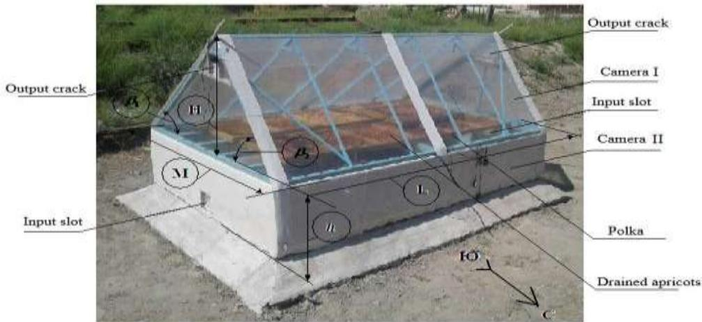
Fig. 1. Experimental direct type solar dryer.
