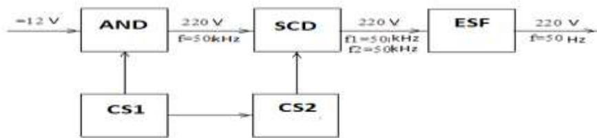
Figure 1. Block diagram of a high efficiency inverter
