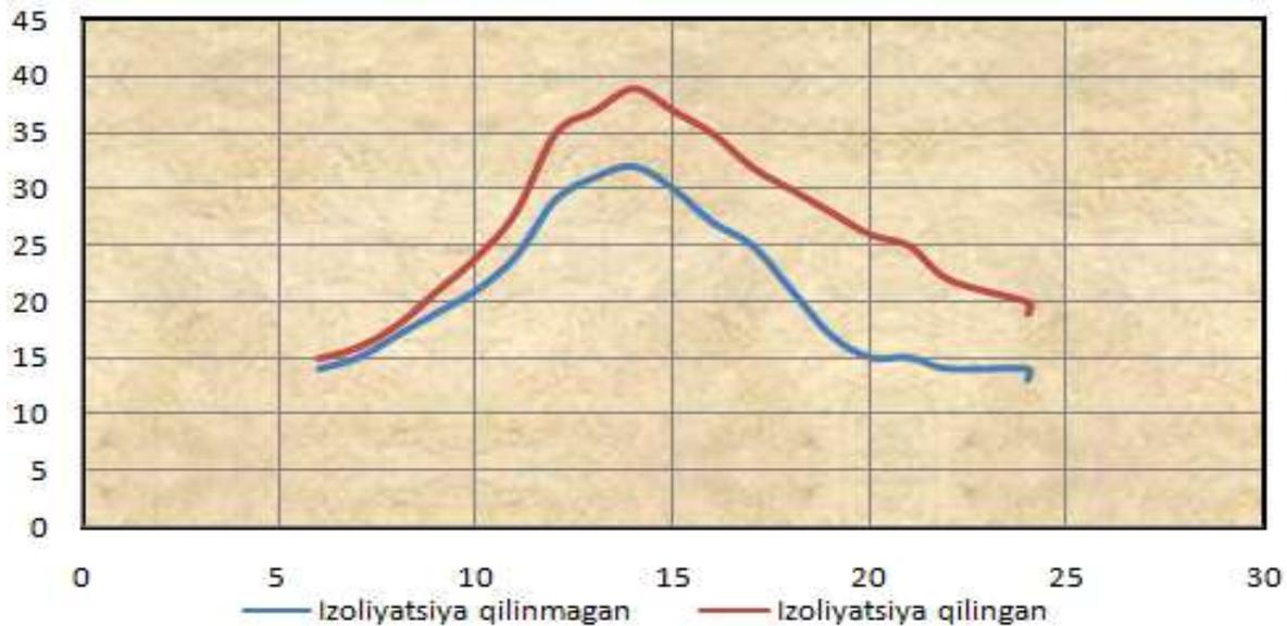
for 24 hours with thermally insulated, aerodynamically operated collector, and thermally insulated and non-aerodynamically collected collectors are shown in the following graph. The graph shows the temperature on the Y axis from  $0^{\circ}$ ....  $+45^{\circ}$ degrees. 0-30 hours on the X axis.
