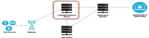
Figure 1. LoRaWAN Network Architecture
