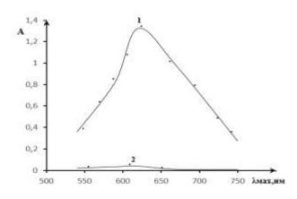
Figure 3. Absorption spectrum of organic amido black reagent immobilized on PPD-1 fiber (l=620 nm): before immobilization (1), after immobilization (2)
