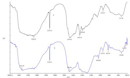
Figure 7. Reagent immobilized on fiber (1) and its complex with lead (2), IR spectra.
