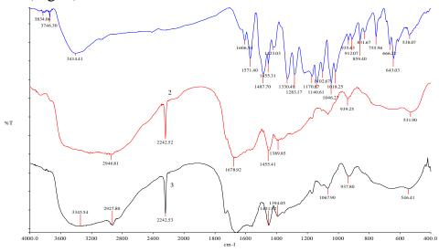
Figure 6. IR spectra of Amido black 10B (1), reagent immobilized on fiber (2), synthetic fiber (3).
