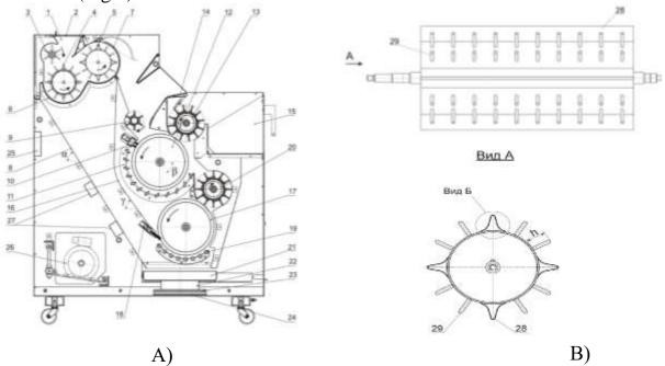
**Figure 1.** Scheme of the improved device for determining the clogging of raw cotton LKM-3. A) -general view of the installation; B) - scheme of the pole-plank drum for cleaning from fine trash
