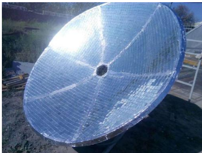
Fig. 3 Appearance of the fabricated parabolic concentrator
