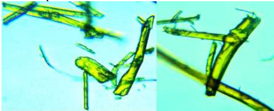
Fig.8. The image of the particles of the "HF" holding silver nanoparticles (1000-fold magnified picture on the microscope "Optika_B-150 DBR")
